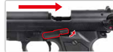
Pull the slide backwards then release.
